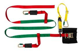
The easy-to-install BuckIt<sup>™</sup> Restraint System keeps the user secure in the bucket, while allowing freedom to move and work. The BuckIt<sup>™</sup> Restraint system features 10,000 lb. rated nylon webbing and can be used with any two dee ring belt, including arborist saddles. The system will fit single-man and man-anda-half buckets. To purchase a belt with the BuckIt<sup>™</sup> Restraint System, please order part number 3852Q8.
